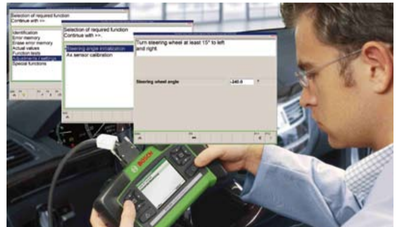
Calibrating the Steering Angle Sensor with a KTS 200
